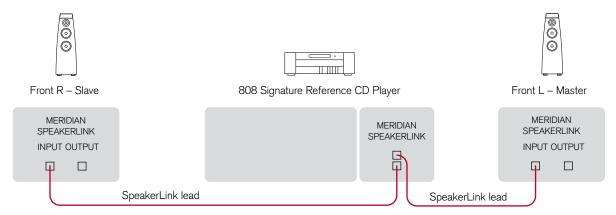
The 808 can be connected directly to Meridian DSP loudspeakers to create a complete compact stereo system, with volume and other preamplifier controls provided by the loudspeakers via the MSR+ or the front panel.
