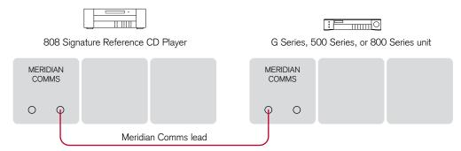
In a system of Meridian products, one of the products acts as the controller for the system, receiving infra-red commands from the MSR+ and then, if appropriate, relaying them to the other products via the Comms link.
