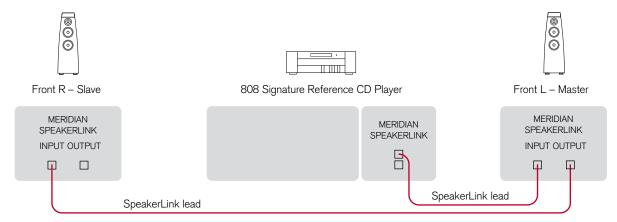
The 808 can be connected directly to Meridian DSP loudspeakers to create a complete compact stereo system, with volume and other preamplifier controls provided by the loudspeakers via the MSR+ or the front panel.
