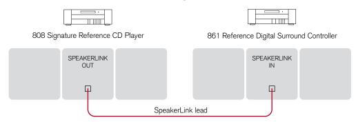
Connect the SpeakerLink output from the 808 to the SpeakerLink input on the 861, using a SpeakerLink lead.
