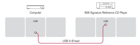
You can connect the 808 Signature Reference CD Player to a PC or Macintosh USB socket to allow you to use the 808 as a digital audio output device.
